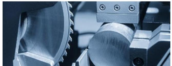
In the event of a power failure, continue driving the saw until the saw blade has moved out of the workpiece.
