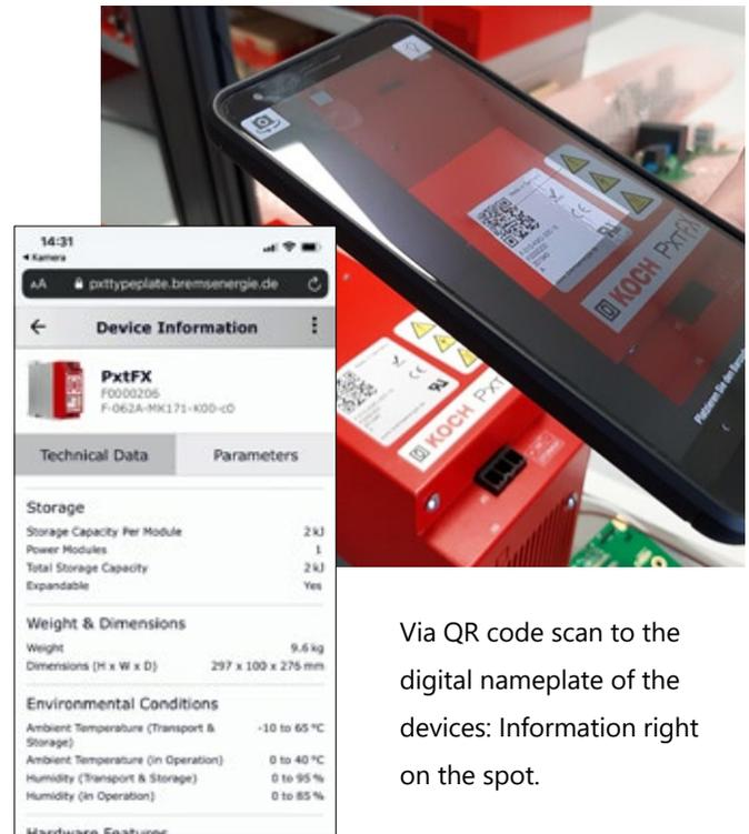
Via QR code scan to the digital nameplate of the devices: Information right on the spot.
