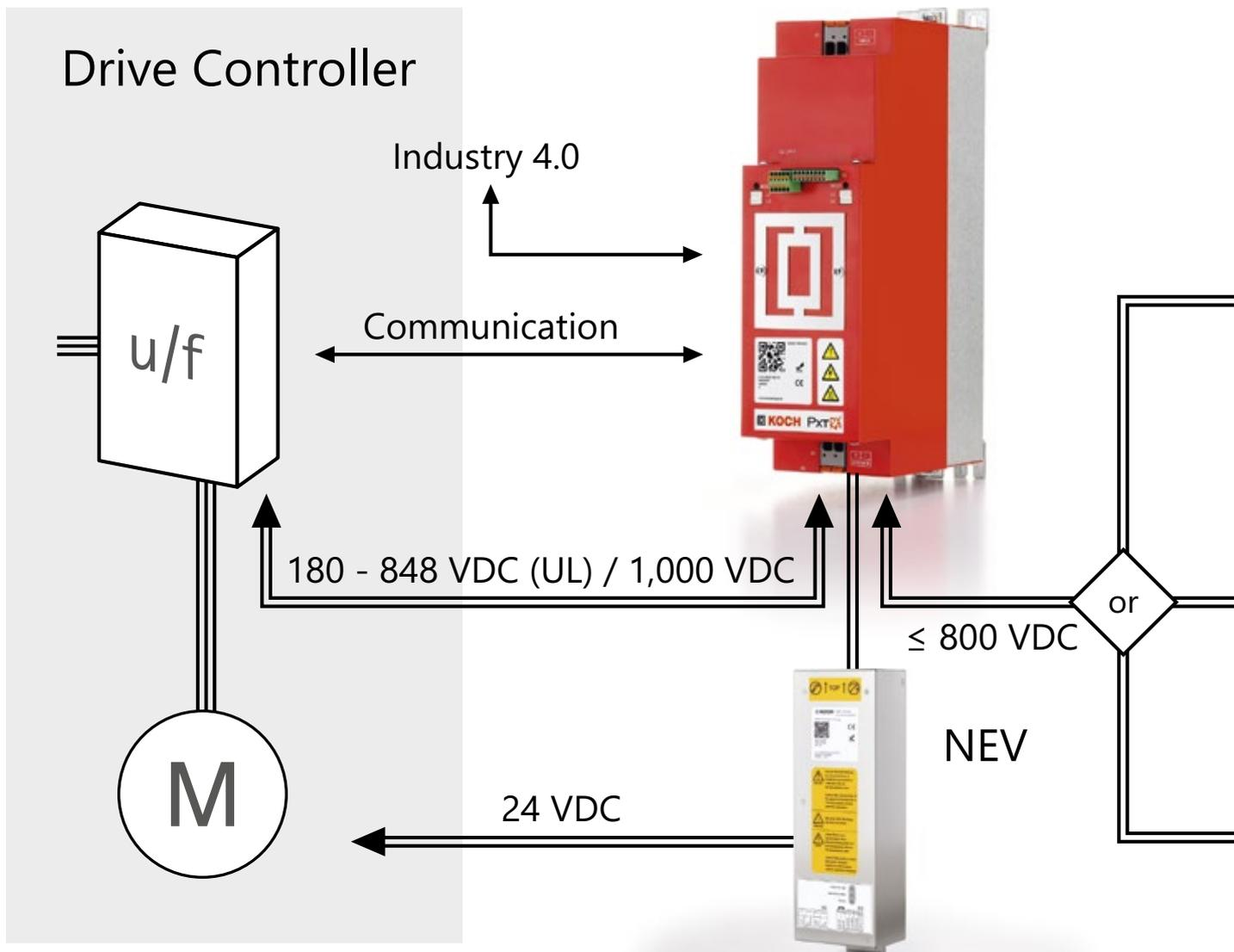
The PxtRX can handle various storage media, which can be selected according to the application and the requirements derived from them. And all this maintenance-free.
