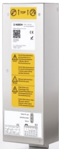
Koch's emergency power supply. The NEV is used to supply electrical power to a 24 V DC circuit independently of the mains.
