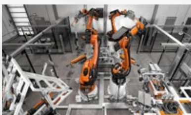
Four robots for welding applications are active together in the cell and use one KTS.
